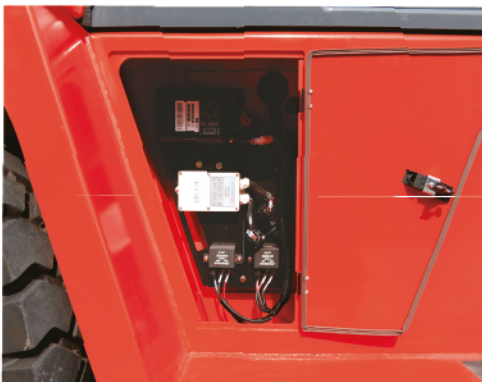
Independent integrated electric cabinet
